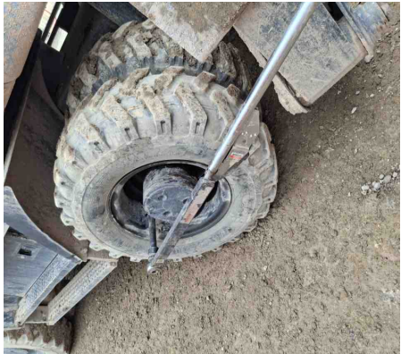
Wheel Position: B2 - Torque 600.0 Nm
