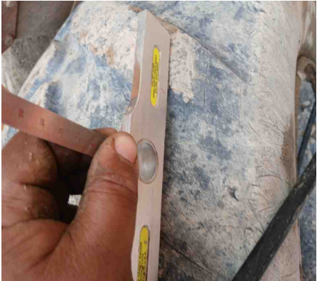
Wheel Position: B2 - Tread Depth Gauge
