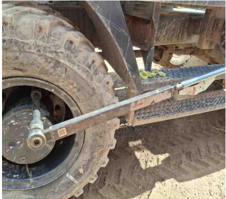
Wheel Position: B3 - Torque 600.0 Nm
