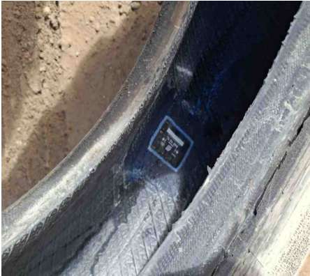
Wheel Position: B4 - Completed Repair
