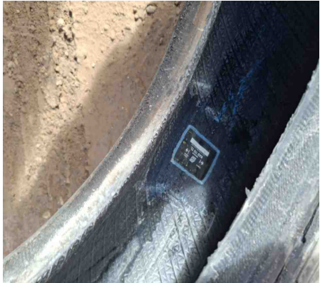
Wheel Position: B4 - Damage Size
