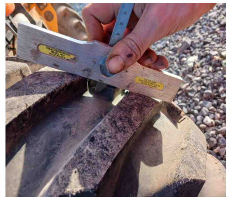
Wheel Position: A2 - Tread Depth Gauge
