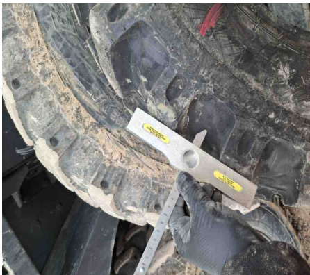
Wheel Position: B2 - Tread Depth Gauge
