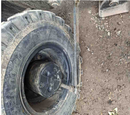
Wheel Position: A2 - Torque 600.0 Nm
