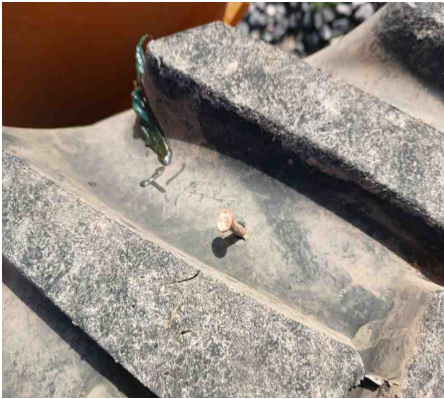
Wheel Position: A2 - Damage Size
